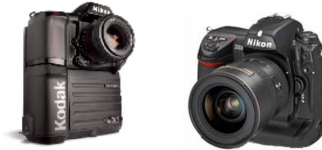
Figure 16. Small-format digital cameras: Kodak DCS 420 (1524x1012 pixels), and Nikon D2x (4288x2848)
