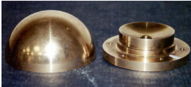
Figure 3. Semi-sphere and cup, main components of the spherical air-bearing
