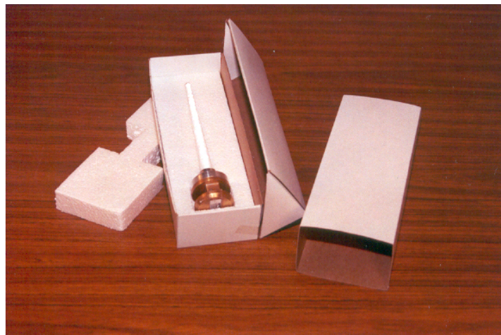
Figure 9. Dielectric antenna and its packaging
