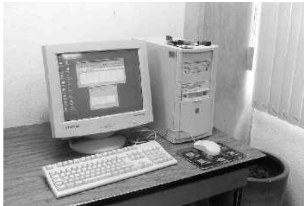
Figure 11. Host computer running the user interface software and acquiring data from RF receiver station
