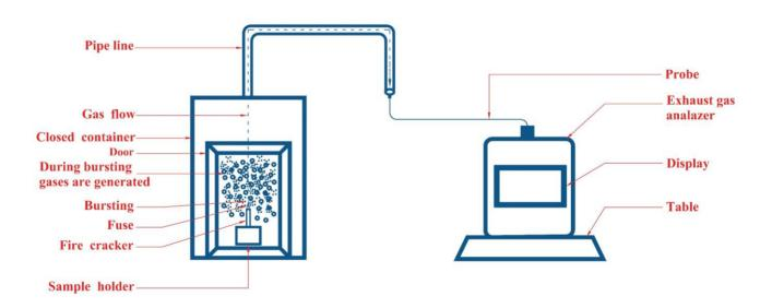
Figure 2a. Experimental setup block diagram.
