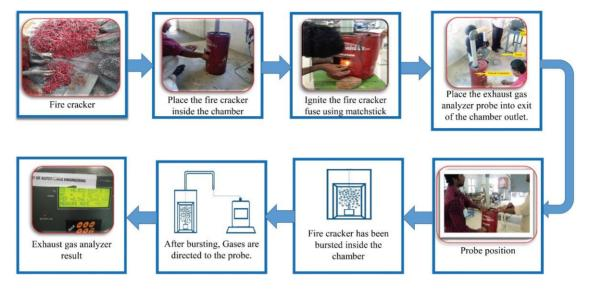
Figure 1. Various processes of emission testing.
