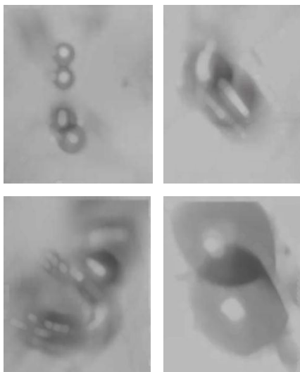
Figure 1. Examples of images of air bubbles captured without a stroboscopic light. Each one of these images show one bubble in motion, appearing as two overlapped or separated objects.
