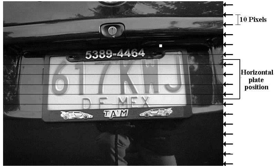
Figure 14. Estimation of matrix B(n,k) used to horizontal plate position estimation. Upper boundaryline plus 5 pixels and lower boundary, line minus 5 pixels
