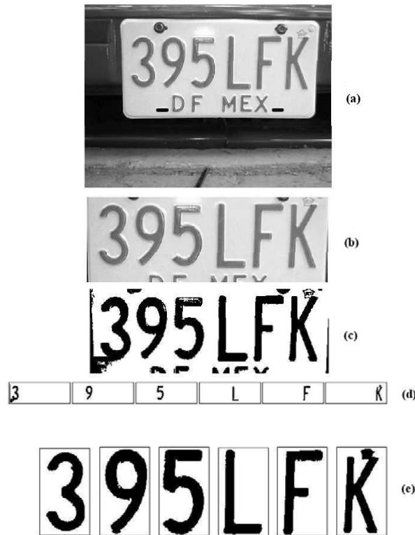
Figure 19. (a) Original image. (b) Automatically localized plate image, using the proposed method. (c) Binary representation of plate image shown in (b). (d) Labels corresponding to the symbols plate after the noise elimination process. (e) Segmented symbols.
