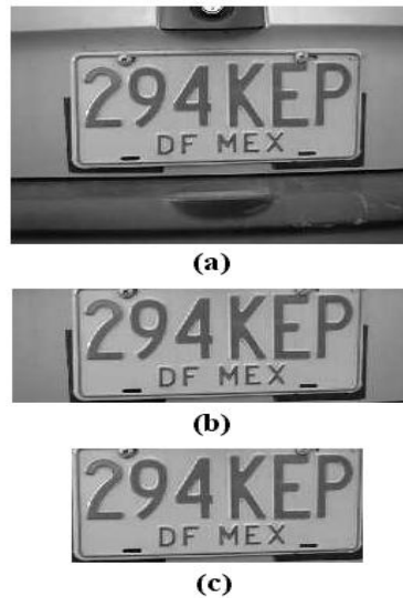
Figure 17. Vehicle plate position estimated using the proposed algorithm. a) Captured image, (b) Horizontal plate localization, (c) Localization process result.
