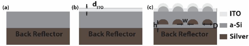
Fig. 1. Cross-sectional view of the device a) bare a-Si with Ag back reflector, b) ITO/a-Si/Ag back reflector, c) Hemispherical nanoparticle for plasmonic behavior (ITO/a-Si (hemispherical Ag nanoparticle)/Ag-back reflector).
