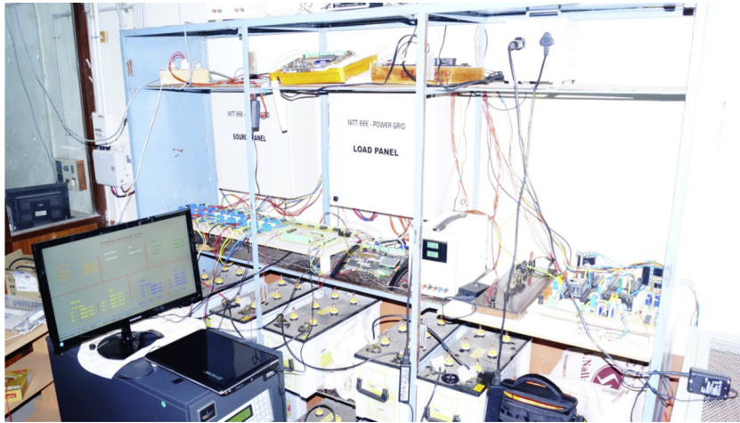
Fig. 6. Hardware setup of the micro-grid with proposed embedded platform.
