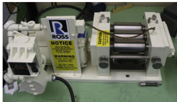
Fig. 1. Ross three-roll-mill used to make CNT-grease.
