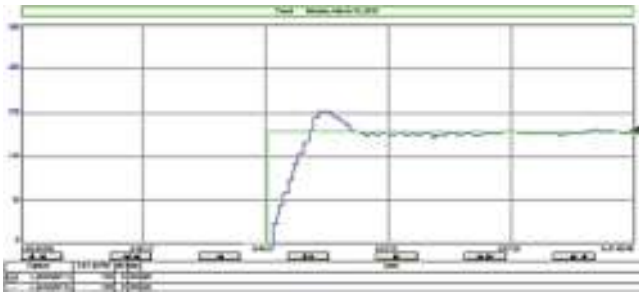
Fig. 14. Performance of Shams tuning IMC-PID controller for the setpoint at 180 lph.
