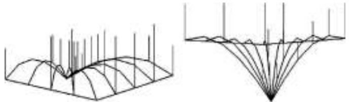
Fig. 7. Final geometry obtained for \{q\}^t = \langle 1 \rangle^{53} using the N-FDM algorithm in Maple®.
