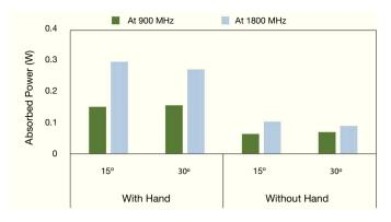
Fig. 4. Total absorbed power for tilt positions (16 mm).
