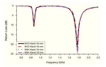
Fig. 10. Return loss curves for 15° tilt positions.
