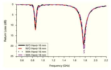
Fig. 7. Return loss characteristics for cheek positions.
