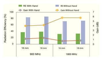
Fig. 6. Gain and radiation efficiency for cheek positions.
