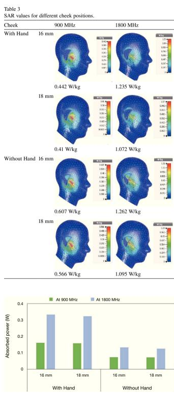
Fig. 3. Total absorbed power by head for different cheek position.
