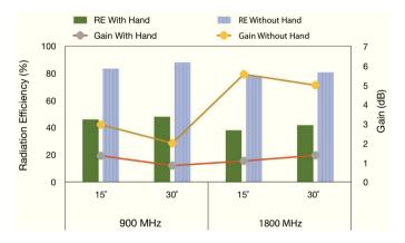
Fig. 9. Gain and radiation efficiency of tilt positions (18 mm).
