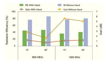
Fig. 8. Gain and radiation efficiency for tilt positions (16 mm).
