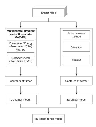
Fig. 1. System architecture.
