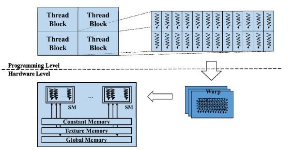
Figure 2. The concept of prgramming and execution in CUDA.
