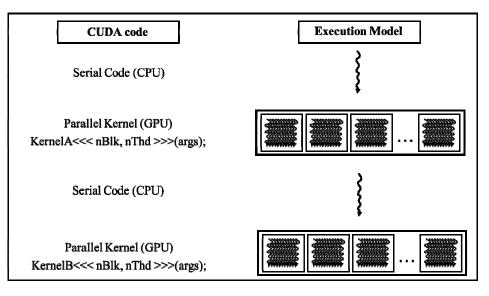
Figure 3. Programming and execution model of CUDA.
