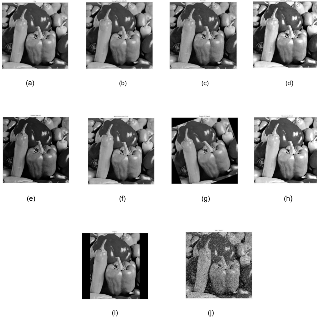
Figure 4. a. Filter (31.7115 dB), b. Scaling 512x512→256x256 (30.4856 dB), c. Gaussian (30.0589 dB), d. Histogram (18.6076 dB), e. Gamma Correction (18.3488 dB), f. JPEG Compression (Q=25) (8.0828 dB) g. Rotation (20 degree) (10.0352 dB), h. Intensity Adjustment (18.7548 dB), i. Cropping (12.8781 dB), j. Salt & Pepper (12.0598 dB).
