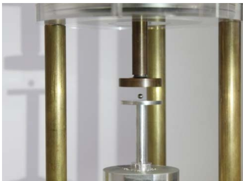
Figure 10. This photograph shows a metal sphere of 3.2 mm in diameter levitated at around 3mm above the radiating disk
