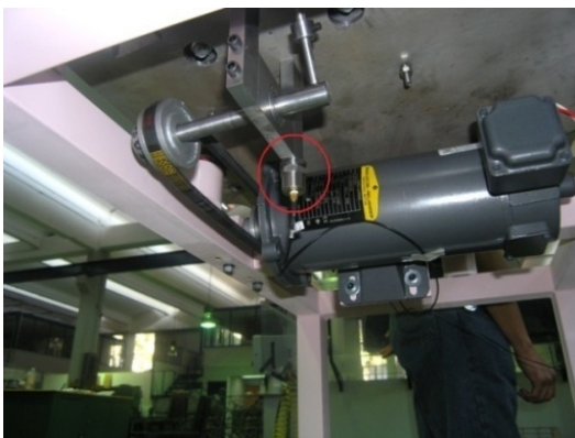
A) Accelerometer below the base of the anti-vibration support system
