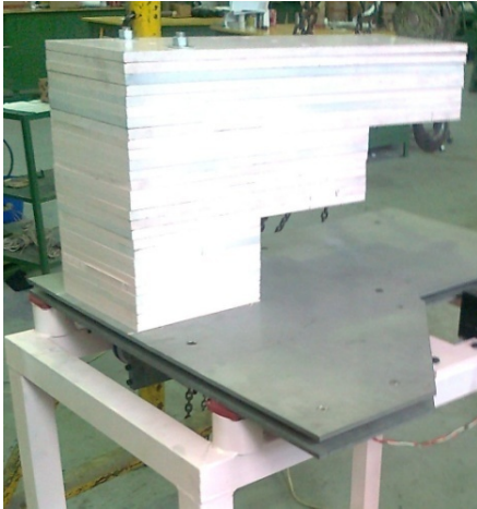
Figure 9. Steel plates simulating mammography equipment weight (250 kg)
