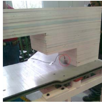
B) Accelerometer above anti-vibration support system
