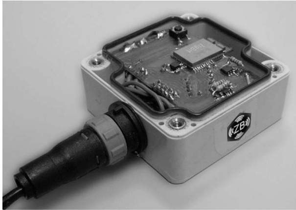
Figure 4. Uncovered module with the circuit board and external connector to the sensors.
