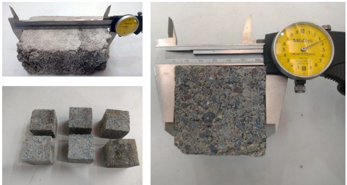
FIGURE 4. Three images showing the preparation process of the piece, in 2020. To acquire the compressive strength, a load was applied at a constant speed and parallel to the longitudinal direction of the specimen, recording the maximum load at failure (Fult), like what has been done by other researchers (Photographs: Alejandro Leal & Alberto Muciño, 2021; source: Authors' Collection).
