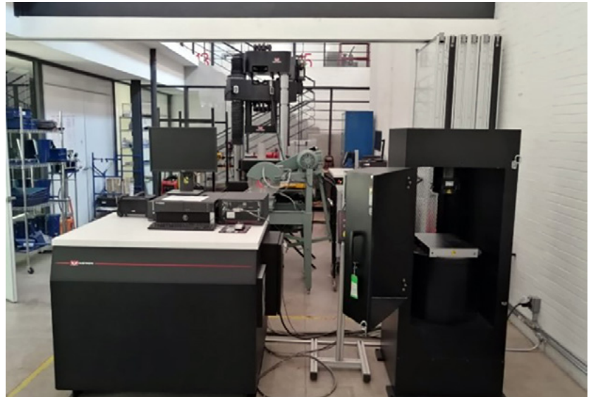
FIGURE 5. Instron® compression testing machine, model 400RD, capacity 200 t (Photograph: Alejandro Leal & Alberto Muciño, 2021; source: Authors' Collection).
