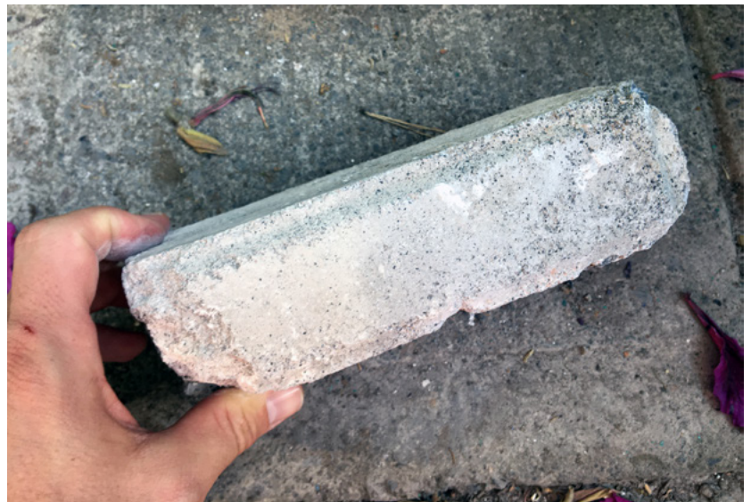
FIGURE 3. Sample of a cement partition wall (20 x 10 x 6 cm) smooth and with bevel, extracted in 2020 from the facade of the house located at Pomona No. 38, col. Roma Norte (Photograph: Alejandro Leal & Alberto Muciño, 2020; source: Authors' Collection).
