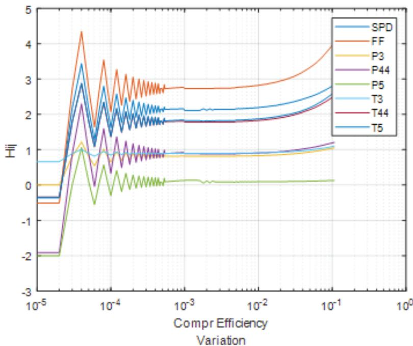
Figure 4. Selection of the optimal value of the compressor efficiency variation (turboshaft)
