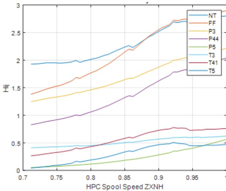
Figure 9. HPC efficiency influence coefficients vs HPC spool speed (turbofan)
