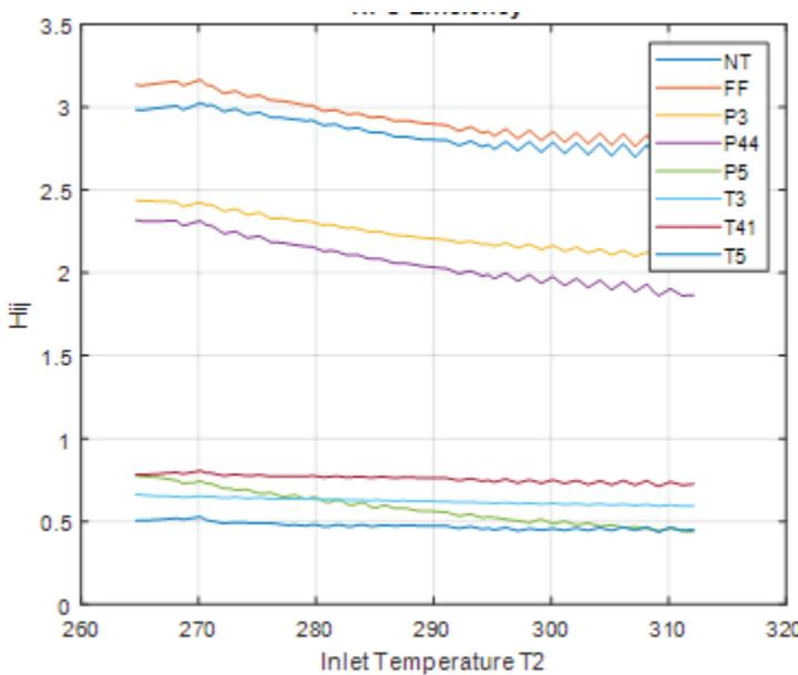
Figure 10. HPC efficiency influence coefficients vs input temperature (turbofan)
