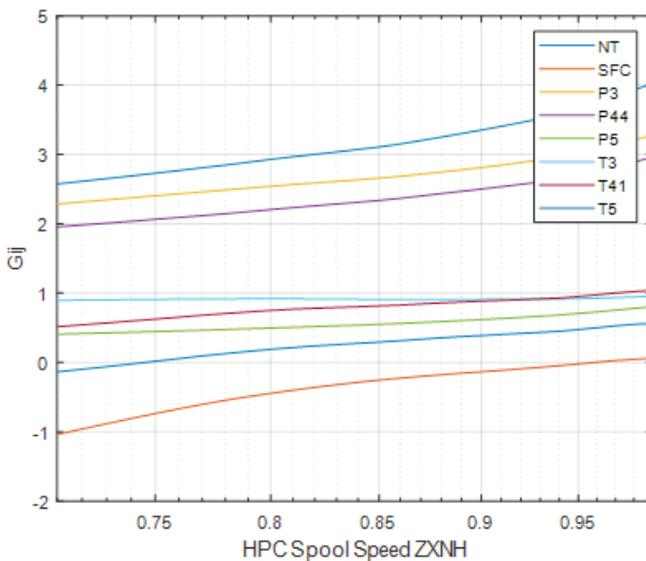
Figure 16. Influence of HPC spool speed on the matrix G coefficients for the turbofan
