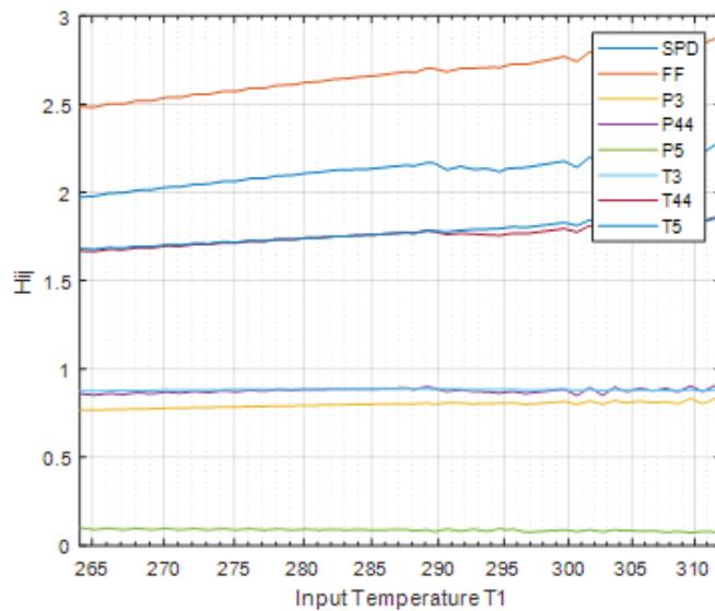
Figure 8. Compressor efficiency influence coefficients vs input temperature (turboshaft)
