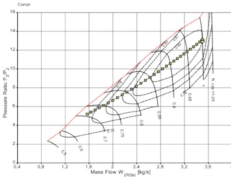
Figure 6. Turboshaft simulated operating points (GasTurb GmbH, 2015)
