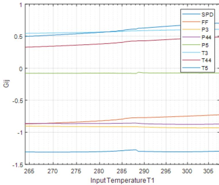
Figure 17. Influence of input temperature on the matrix G coefficients for the turboshaft
