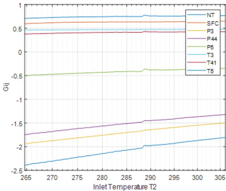
Figure 18. Influence of the input temperature on the matrix G coefficients for the turbofan
