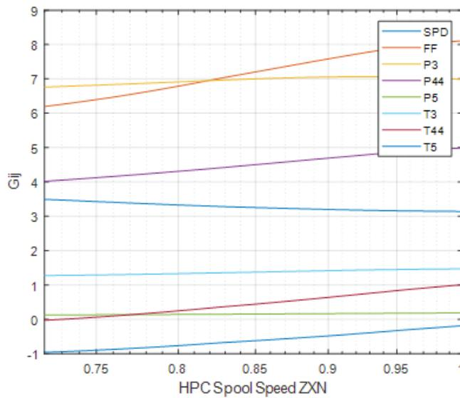
Figure 15. Influence of HPC spool speed on the matrix G coefficients for the turboshaft
