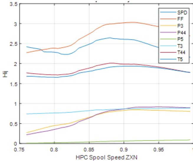
Figure 7. Compressor efficiency influence coefficients vs HPC spool speed (turboshaft)
