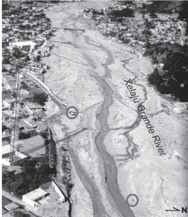
Figure 12. View from the east of the Xelajú Grande River showing the damage caused by the Hurricane Stan in October 2005. The source materials of the flow event were originated in high lands located westward of Motozintla. The debris flow deposit shows frontal lobes and levees. Red circles point out a person and a heavy duty truck.
