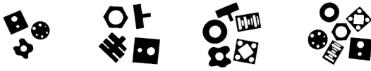
Fig. 3. Binary images of 320 \times 240 pixels with a different number of objects of diverse complexity used to test the performance of the trained perceptron to estimate the Euler characteristic of a 2-D binary image
