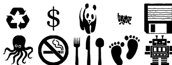
Fig. 2. Binary images of 128 \times 128 pixels of ten different logos used to test the performance of the trained perceptron to estimate the Euler characteristic of a 2-D binary image
