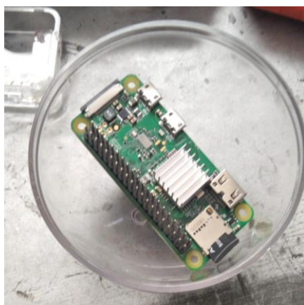
Fig. 14. shows a Raspberry Pi Zero inside an acrylic sphere of approximately 8 cm diameter
