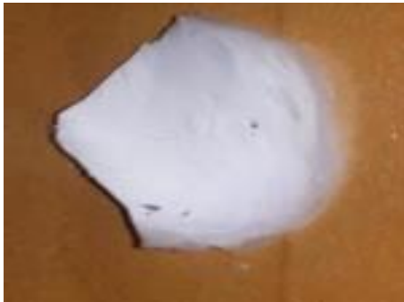
Fig. 2. Fiber mats produced by electrospinning machine
