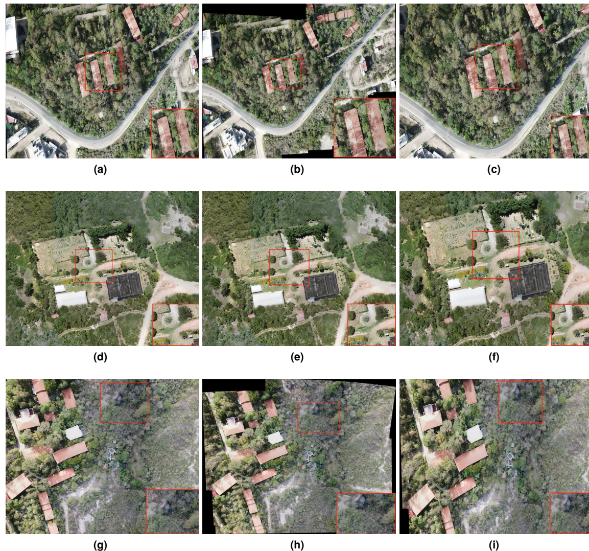
Fig. 1. Results comparison. The images in the first column show the orthomosaics obtained by means of a manual reconstruction carried out by an expert. The orthomosaic obtained with our methodology shown in the second column. The last column shows the reconstruction obtained with the Pix4DMapper software
