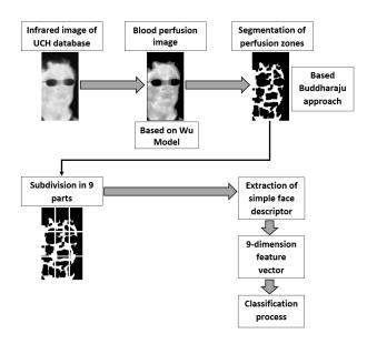
Fig. 1. Diagram of our thermal face recognition process
