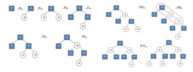
Fig. 9. A step by step insertion algorithm
