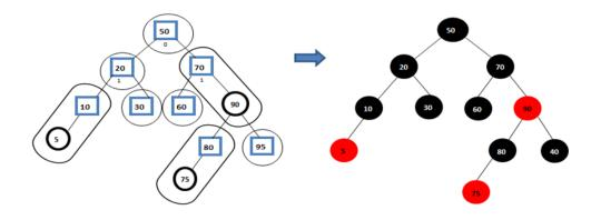
Fig. 4. The new structure as a Red-Black tree
