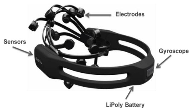
Fig. 3. Device used for acquiring the EEG signals
