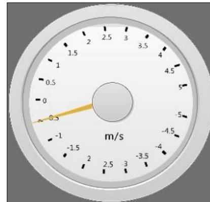
Fig. 6. Vertical speed indicator
