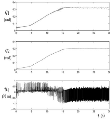
Fig. 4. Position and control of the torsional system
