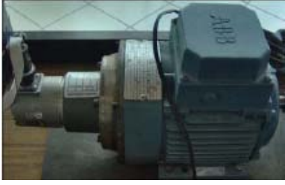
Fig. 4. Encoder coupled with the induction motor
