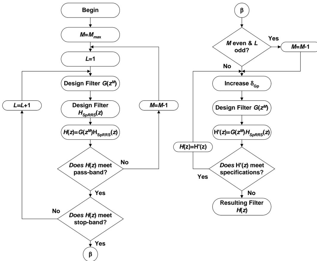
Fig. 3. Flow diagram of the proposed algorithm.
