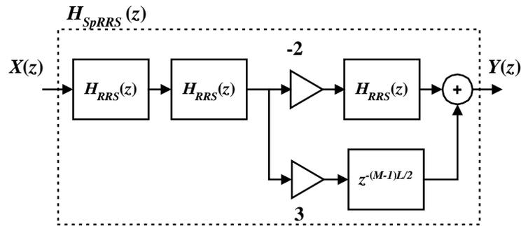
Fig. 2. Sharpening polynomial structure for  $\sigma = \delta = 0$  and  $n = m = 1$ .
