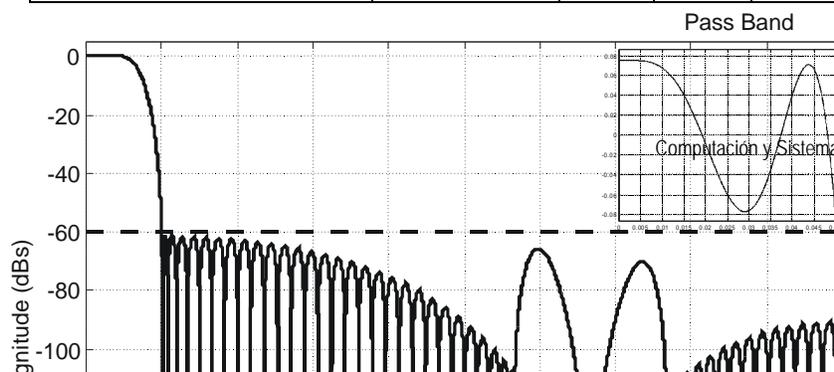
**Fig. 4.** Design example magnitude response obtained with the proposed algorithm with sharpening polynomial parameters  $\sigma = \delta = 0, m = n = 1$ .
