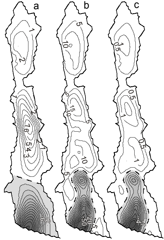
Figure 2. Streamfunctions in Sv of the integral circulation for (a) planetary, (b) topographic and (c) effective barotropic background currents in the Gulf of California. The efficiency parameter \alpha for (c) is 0.07. Darkened areas correspond to cyclonic circulation.
