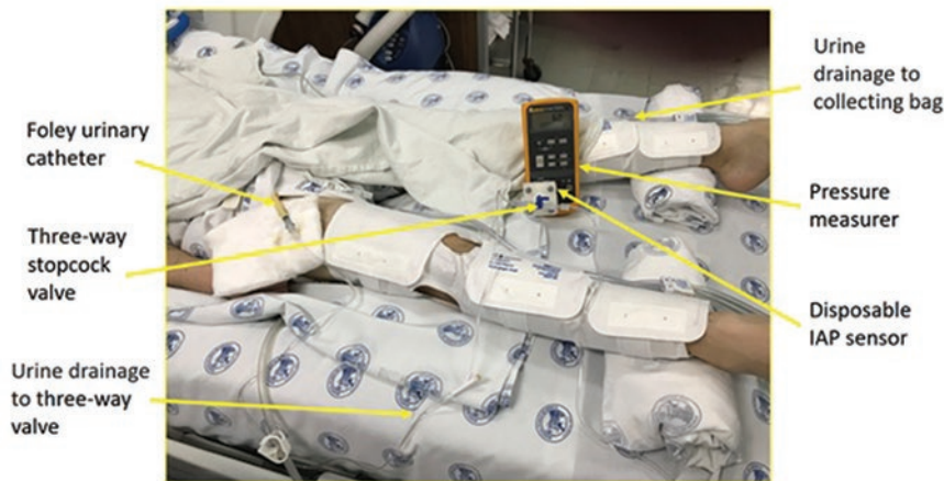
Figure 3. Measure of intra-abdominal pressure in a patient using the proposed disposable transducer.
