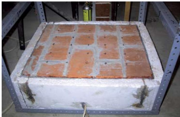
**Figure 2: A red brick wall mounted on the testing prototype.**
