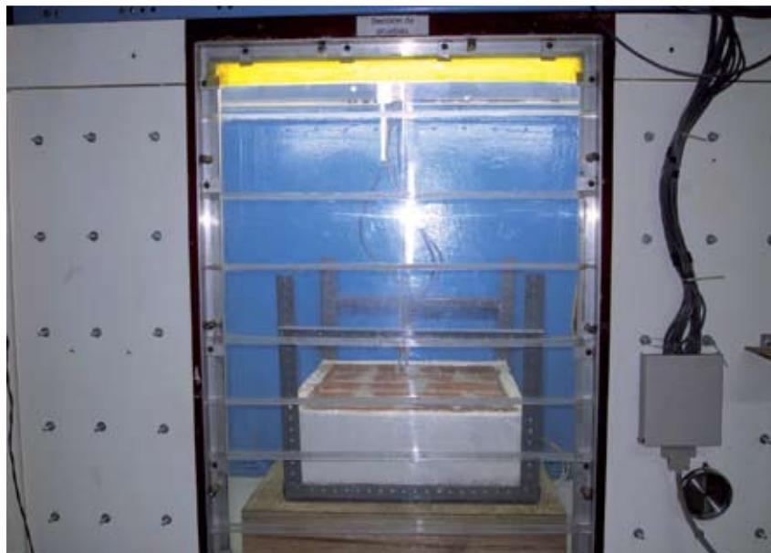
**Figure 4: View of prototype testing within the test section of the wind tunnel.**
