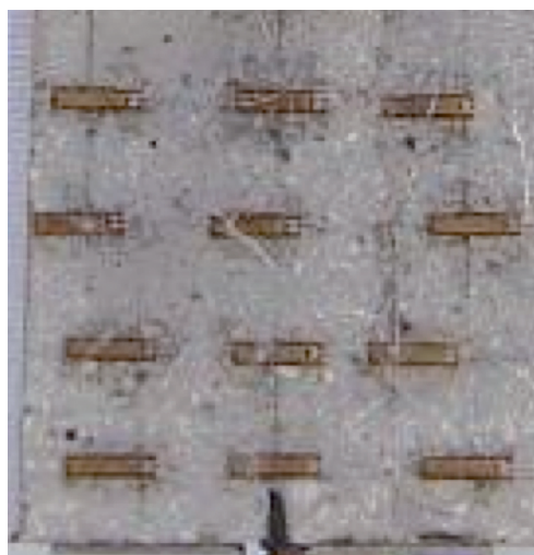
Fig. 2. Arrangement of stain gauges.
