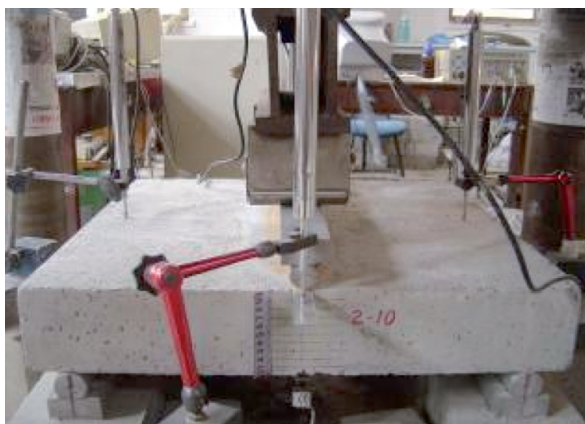
Fig. 3. Set up of the panel test.
