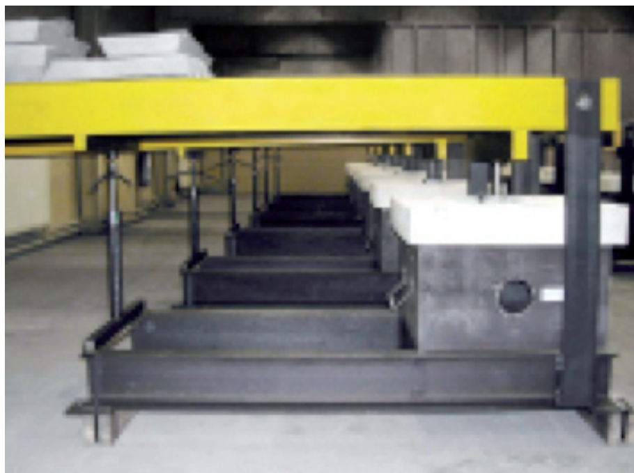
Picture 7: Creep test set up.
