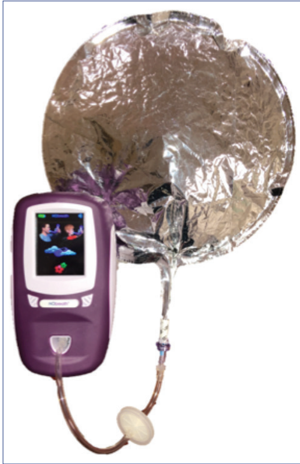
Figure 2. Mylar® bag connected to the sampling line and the electrochemical device.
