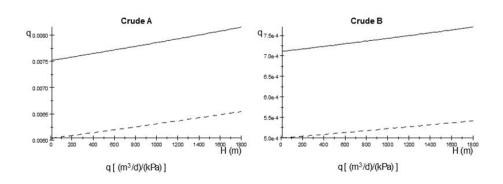
**Figure 4.** The behavior of the quotient (q) between crude oil flow (m<sup>3</sup>d<sup>-1</sup>) and pressure drop (kPa) at L = 1000 m for distance (H) (m) with an enhancer volume fraction m of 0 (dashed line) and 0.01 (solid line). Source: Authors' own elaboration.
