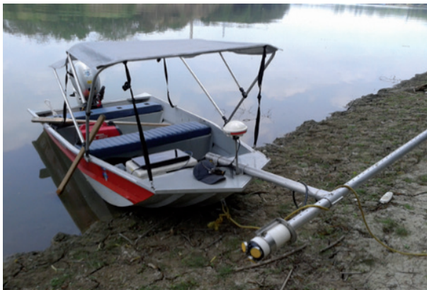
Fig. 5. ADCP, RiverCat and GPS on the boat.
