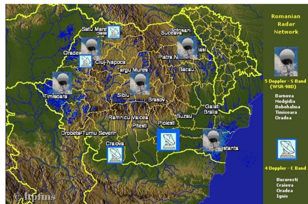
Fig 1. The SIMIN radar network: five WSR-98D S-band radars (an upgraded version of the WSR-88D radar used in the US NWS network) and four C-band radars (two from EEC –DWSR-2500C type and two from Gematronik–METEOR 500C type).
